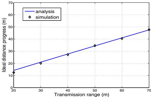
Fig. 3. Ideal distance of a relay node. Average number of neighbors in simulation is 100.
