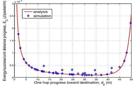
Fig. 1. Normalized energy consumption versus Euclidean distance progress. In simulation, average number of neighbors = 100.
