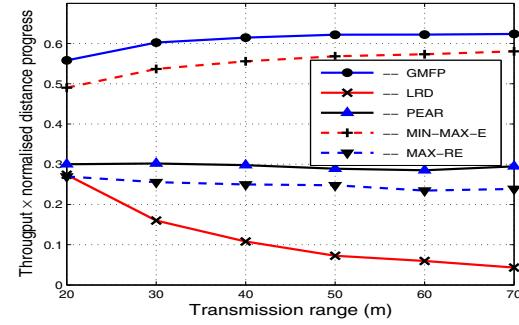
Fig. 4. Fair throughput comparison of different protocols.
