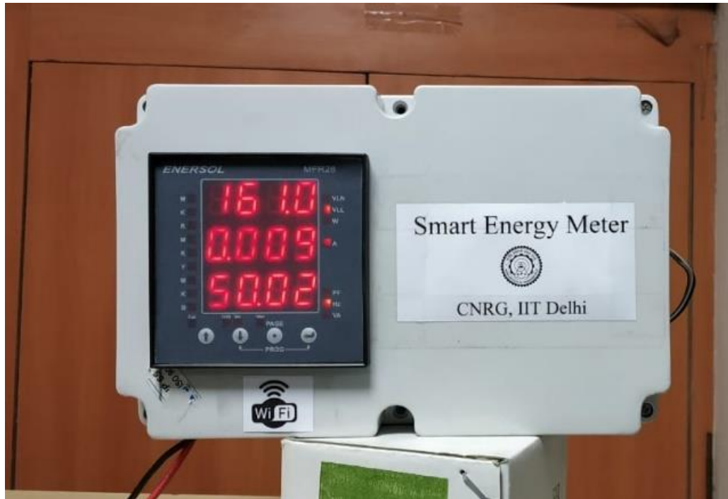
Fig. 6. Smart Energy Meter with Data Pruning Subsystem.
