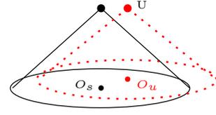
Fig. 1. Depiction of hovering inaccuracy of UAV-aided RFET.
