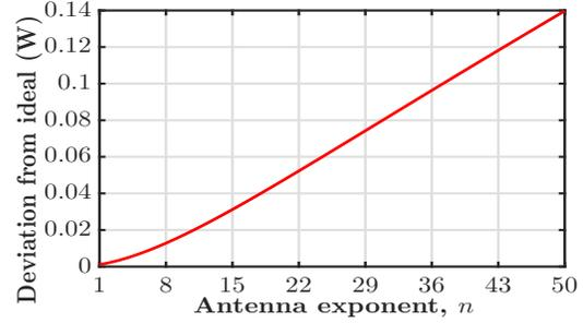
Fig. 3. Deviation in received power against antenna exponent for  $h = 1$  m.
