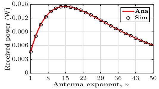
Fig. 2. Variation of received power against antenna exponent for  $h = 1$  m.
