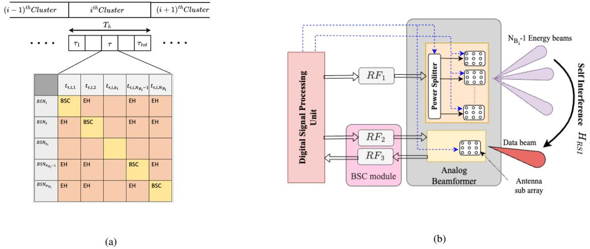
**Figure 2:** (a) Proposed multi-BSN serving protocol: Illustrating the total hovering time  $T_h$  for the  $i^{th}$  cluster with  $N_{B_i}$  BSNs, partitioned into  $\tau_{tot}$  intervals, each interval further segmented into  $N_{B_i}$  slots. (b) Proposed transceiver architecture at the UAV.
