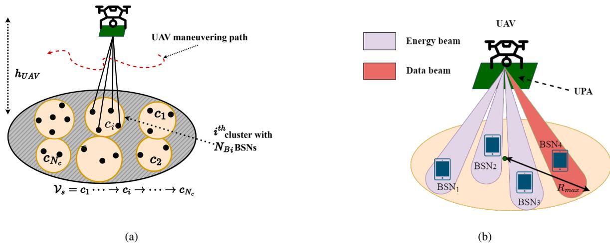
**Figure 1:** (a) Illustration of  $N$  BSNs, grouped into  $N_c$  clusters with  $N_{B_i}$  BSNs in  $i^{th}$  cluster being served by the UAV according to cluster visiting sequence  $\mathcal{V}_s$ . (b) UAV serving  $i^{th}$  having  $N_{B_i} = 4$  BSNs with a total  $N_B = 4 (= N_{B_i})$  beams.
