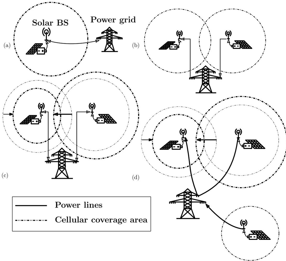
Figure 1: Illustration of (a) isolated grid-connected and renewable energy powered BS (as an example, we use solar power), (b) BS load aware energy sharing, (c) BS green energy aware coverage adjustment based load management, (d) proposed CASE framework for green cellular network services.
